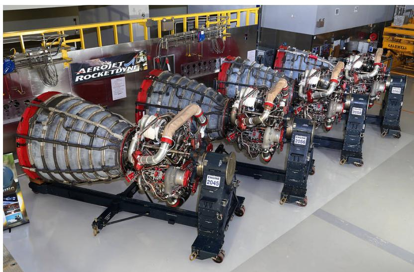
Fig. 13 RS-25 Engines for SLS First Flight ready for Integration with Core Stage
