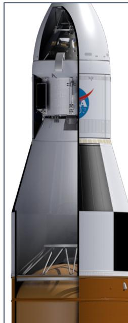
Fig. 7. SLS 8.4 m Diameter Fairings
