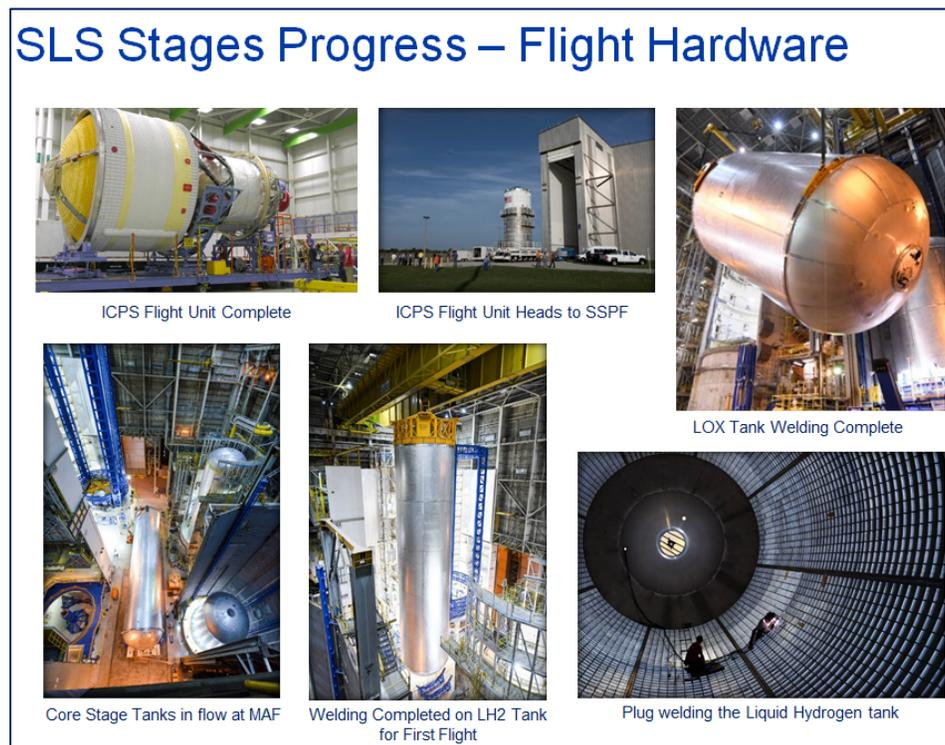
Fig. 9 Montage of SLS Flight Hardware
