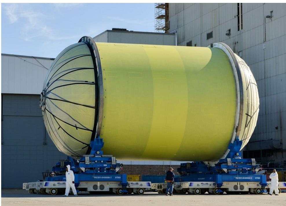
Fig. 11 SLS Core Stage Liquid Oxygen Tank at NASA MAF
