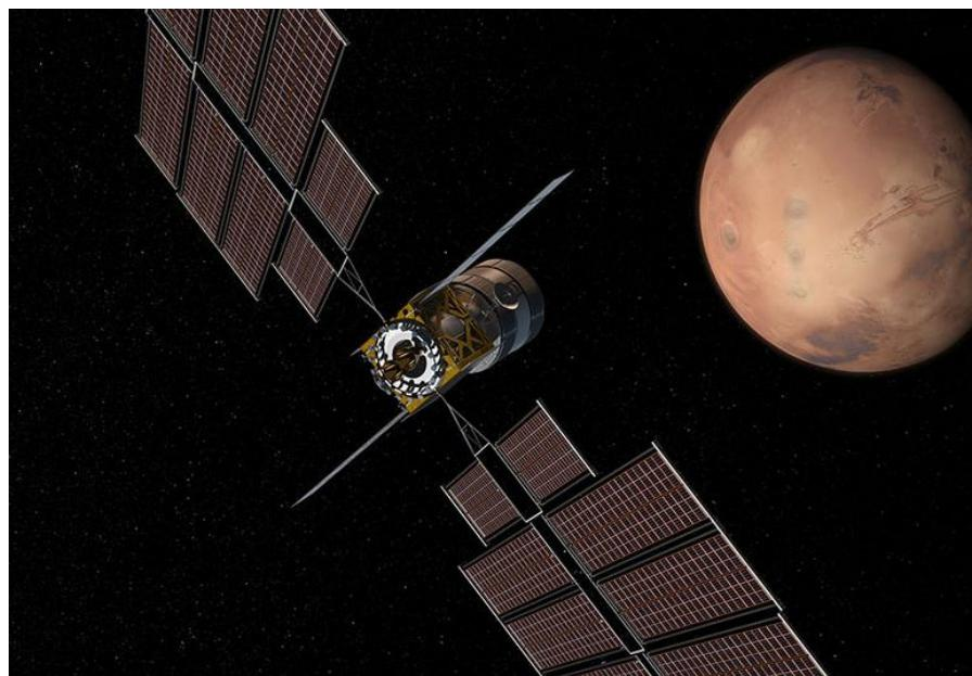
Fig. 41 Solar Electric Propulsion (SEP) Mars Transfer Vehicle
