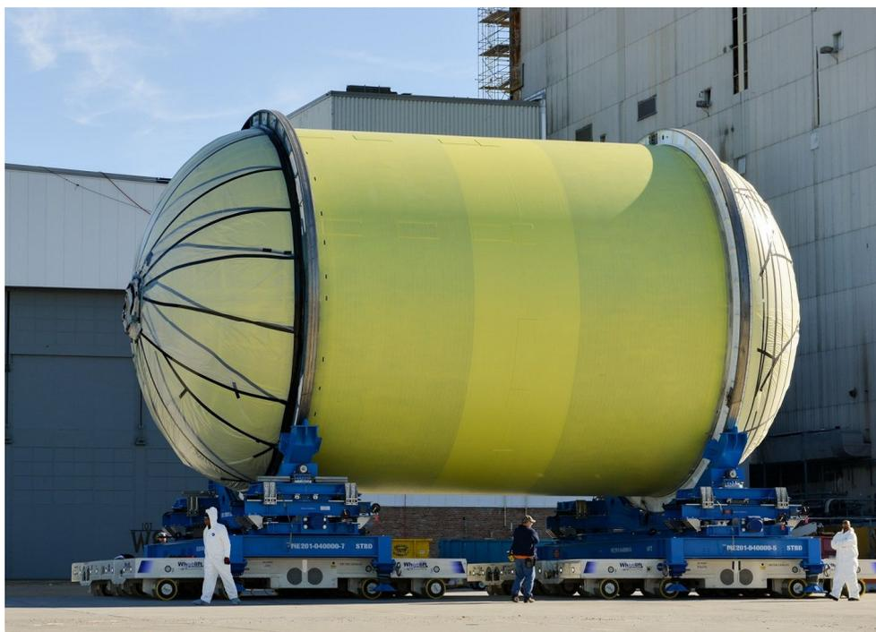
Fig. 11 SLS Core Stage Liquid Oxygen Tank at NASA MAF
