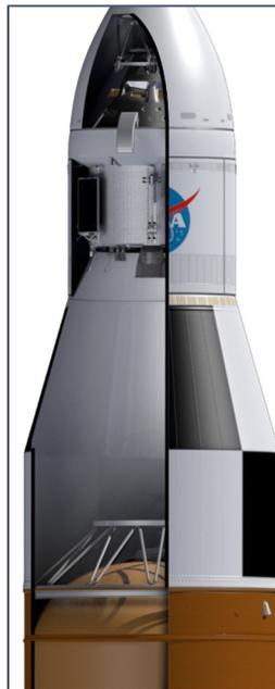
Fig. 7. SLS 8.4 m Diameter Fairings
