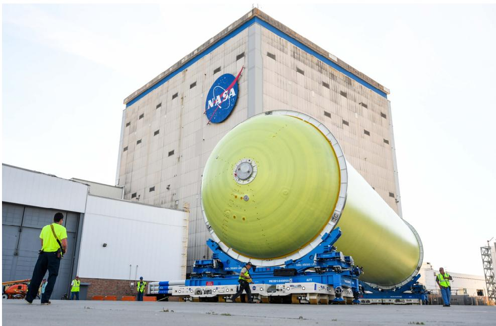
Fig. 10 SLS Core Stage Liquid Hydrogen Tank at NASA MAF
