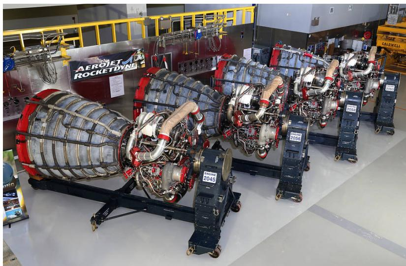
Fig. 13 RS-25 Engines for SLS First Flight ready for Integration with Core Stage (Aerojet-Rocketdyne photo)
