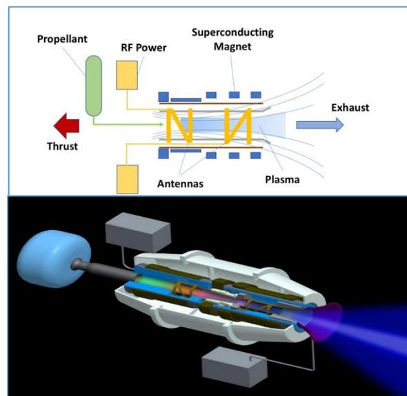
Fig. 3 VASIMR simplified diagram and cutaway.
