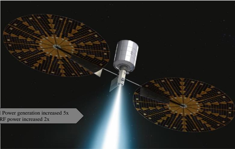
**2021.** 150kW **pulsed** (40kW average) configuration demonstrating NASA HEMOD and DOD Technology goals and DRM1,2,3 objectives.
