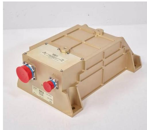
**Fig. 5 270v Li-ion battery energy store.**
