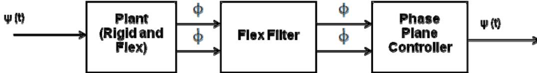
**Figure 1: Dynamics and Control Block Diagram**
