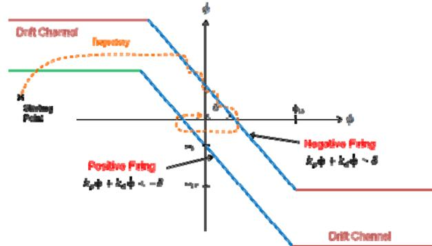
**Figure 2: The Phase Plane Controller**
