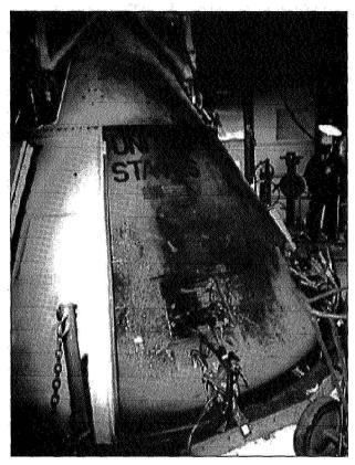
External view of fire damage to the Apollo 1 CM (NASA S67-21295).
