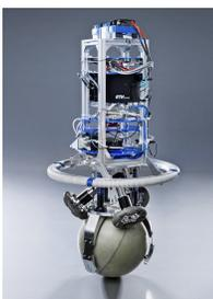
Fig. 11. Ball balancing robot. This robot consists of three major elements: the ball, the propulsion unit and the upper body (torso). The ball is driven by three omniwheels mounted on brushless motors with planetary gear heads. Through optical encoders on the motors, the ball rotation is measured providing onboard odometry for the robot.
