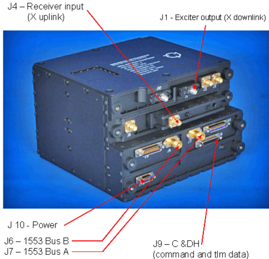
Fig. 8-53. Group III small deep space transponder.
