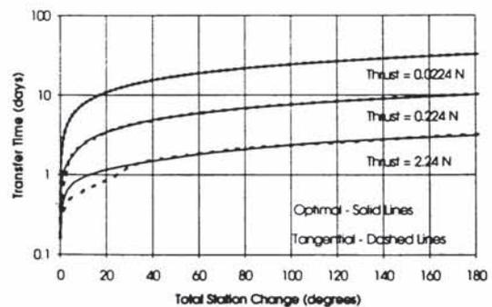
Fig. 2. Optimal Station Change Maneuver
