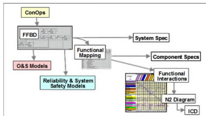
Figure 2. Functional Analysis and Requirements Allocation Process
