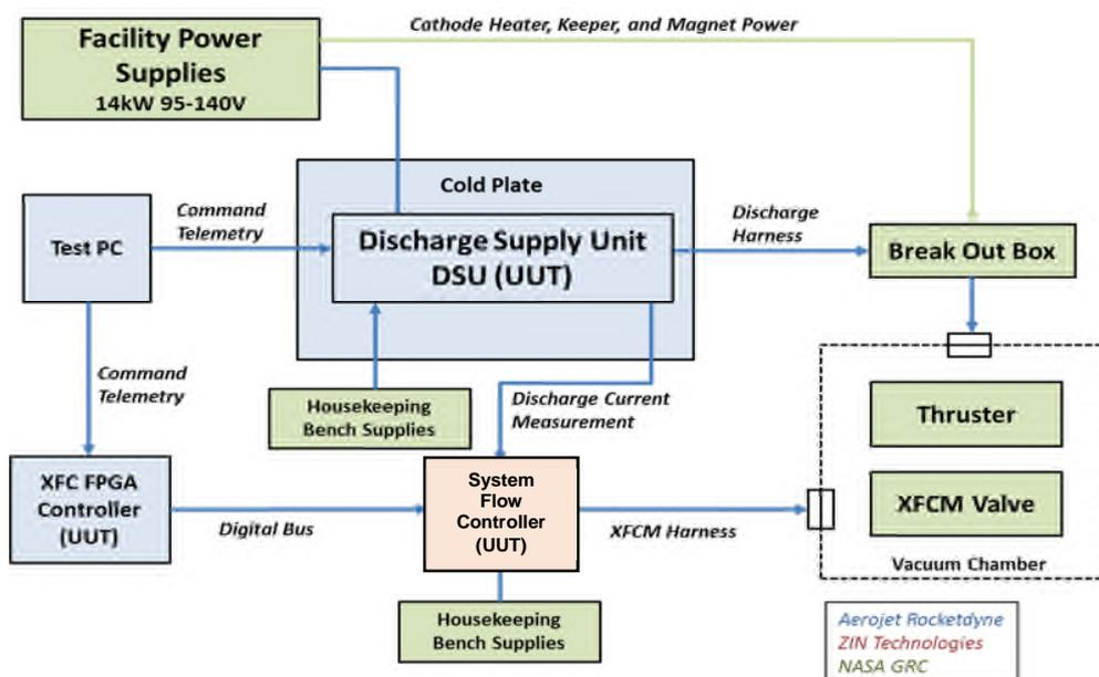
Figure 7. Early Integrated System Test Diagram
