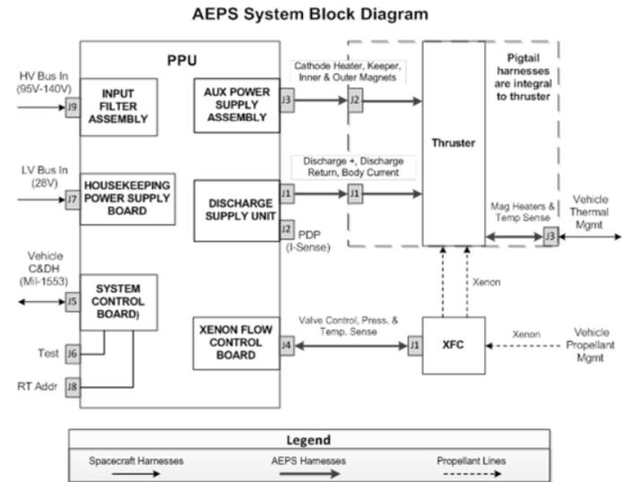
**Figure 4. AEPS Block Diagram with electrical and propellant interfaces**
